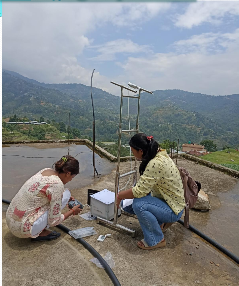
Collection of ambient air using Mercury Monitoring Tool Kit
